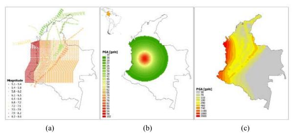
**Figure 1.** (a) Seismic events location included in the analysis (array of epicenters across de seismic faults); (b) Example of the spectral accelerations estimated for a single event; seismic source: "Benioff intermedia", magnitude: Mw 7.75, depth: ≈100km. (c) Hazard map for a 500 years return period (AIS, 2009).
