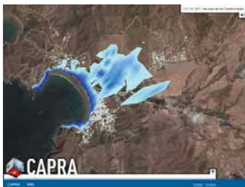
San Juan del Sur, Nicaragua: 500 years return period tsunami run-up height over the coast of the city.
