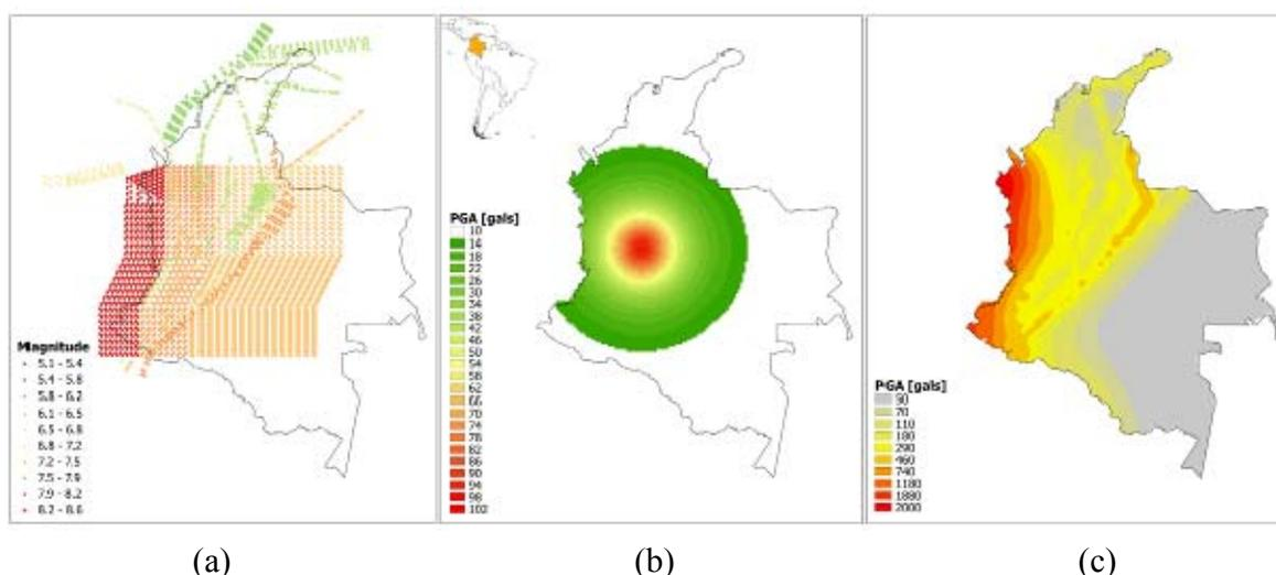
**Figure 1.** (a) Seismic events location included in the analysis (array of epicenters across de seismic faults); (b) Example of the spectral accelerations estimated for a single event; seismic source: "Benioff intermedia", magnitude: Mw 7.75, depth:  $\approx$ 100km. (c) Hazard map for a 500 years return period (AIS, 2009).
