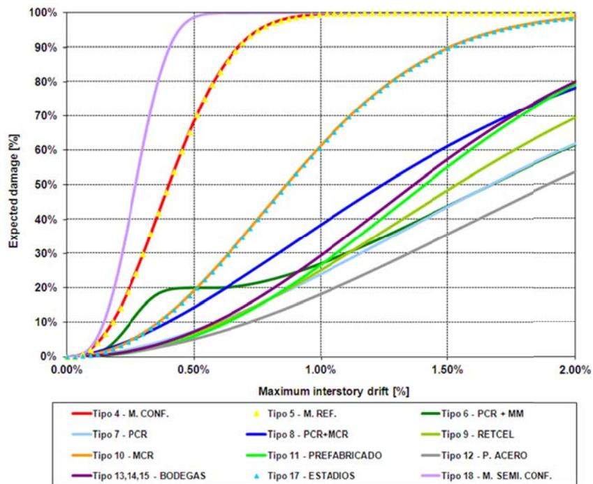
Figure 5. Vulnerability functions based on maximum inter-story drift
