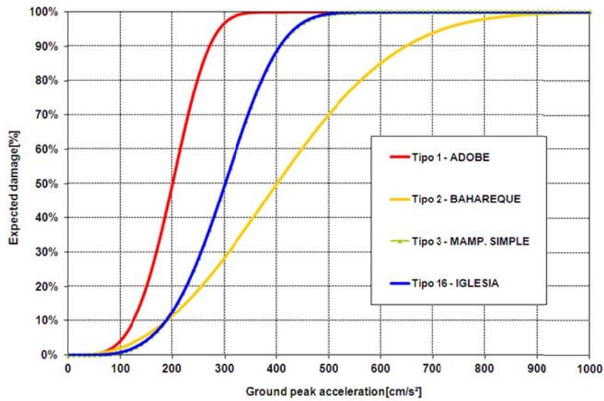
Figure 4. Vulnerability functions based on peak ground acceleration
